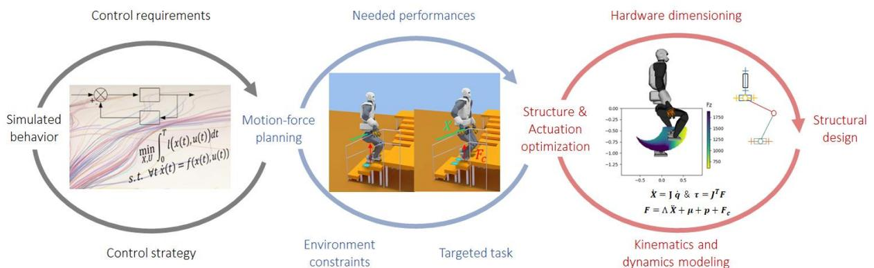
Figure 1. Framework of a mechatronic codesign approach
