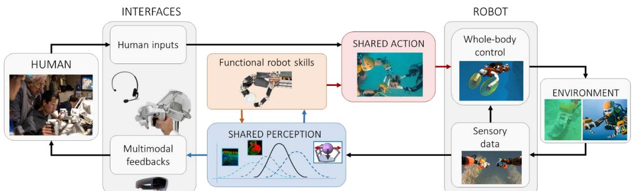
Figure 1. Shared-autonomy framework in haptic teleoperation
