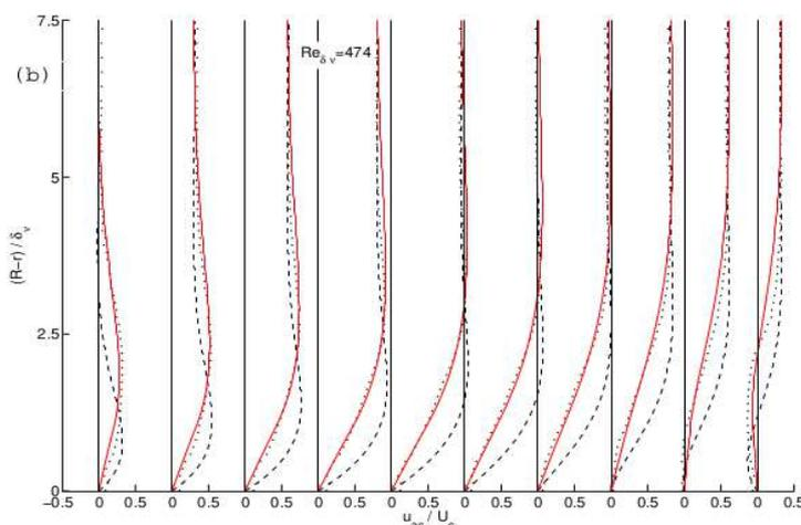
**Figure 1 : Oscillating boundary layer in high level waveguide.**
