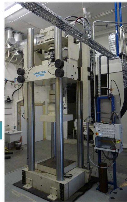
Qualification des performances machine en compression/torsion
